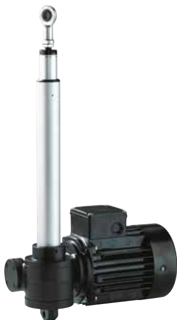
ATEX approved actuator based on a worm gear drive. The actuator is mounted with cylindrical aluminium tubes and an inner threaded spindle
