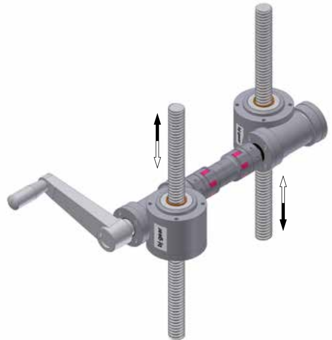
Synchronous movement in two directions with manual operation
